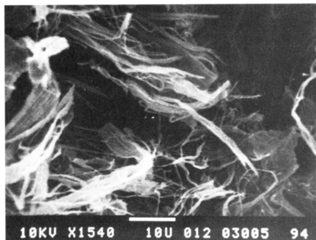
Figure 4. SEM micrograph of the oligo(4'-HBCA) prepared in bulk, 18 h/270 °C (no. 3).
